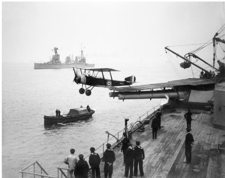
A Sopwith launching from one of Australia 's turrets (Donor Sandra Fox 2007)
